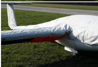
Protective covers Wing and fuselage protective covers protect all exposed surfaces from inclement weather, UV radiation, moisture, dust, and bird droppings. The multi-piece covers join together with Velcro, and are held in place with elastic cords.
