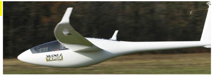
The pylon takes 14 seconds to deploy and the engine can be started almost immediately
