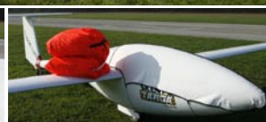
Protective covers Wing and fuselage protective covers protect all exposed surfaces from inclement weather, UV radiation, moisture, dust, and bird droppings. The multi-piece covers join together with Velcro, and are held in place with elastic cords.
