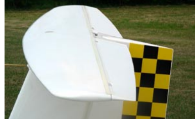
The incidence of the variable-position horizontal tailplane is ingeniously governed by the flaperon setting. The more negative the flap setting, the greater the angle of incidence. The conventional elevator remains in trail resulting in minimal trim drag.
