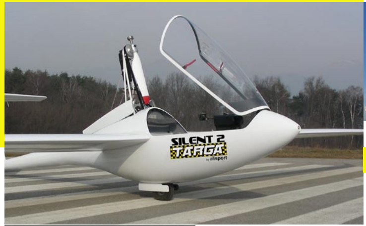
The incidence of the variable-position horizontal tailplane is ingeniously governed by the flaperon setting. The more negative the flap setting, the greater the angle of incidence. The conventional elevator remains in trail resulting in minimal trim drag.
