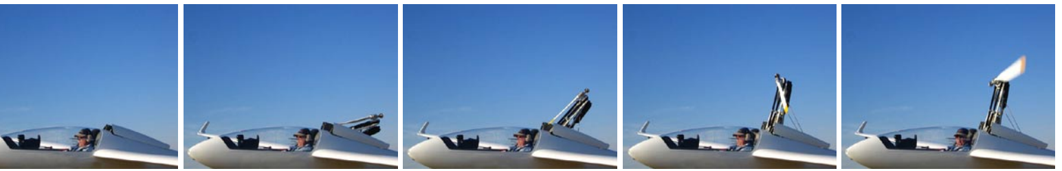
The pylon takes 14 seconds to deploy and the engine can be started almost immediately
