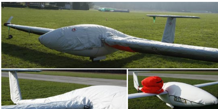
Protective covers Wing and fuselage protective covers protect all exposed surfaces from inclement weather, UV radiation, moisture, dust, and bird droppings. The multi-piece covers join together with Velcro, and are held in place with elastic cords.
