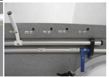
The incidence of the variable-position horizontal tailplane is ingeniously governed by the flaperon setting. The more negative the flap setting, the greater the angle of incidence. The conventional elevator remains in trail resulting in minimal trim drag.
